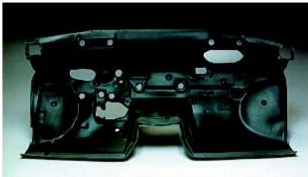
A typical Dash Insulator
