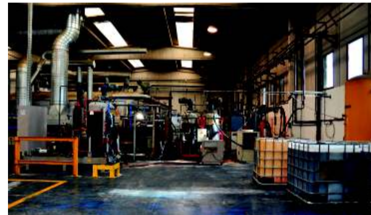
One Cannon piston machine is dispensing the heavily filled formulation, another feeds the second layer of sound absorber, a light flexible foam.
